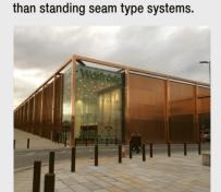
The thickness of the panels is commonly 1mm, with widths up to 333mm and joint widths from 0mm to 20mm and 5mm to 20mm for Zinc. Reveal Panels are normally fixed back to timber or metal sub frames with a pressure equalised, ventilated airspace.
