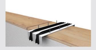
Install angle fixing strips between the Topclip joints with stainless steel annular ring nails or screws.
